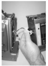
2) Ensure that appropriate power connectors are connected and that the battery gasket is positioned between DR-DV-5000 and camera.
