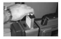
Connect just the FSHDD-1 FireWire HDD to a Macintosh or Windows computer system with an OHCI compliant FireWire port. FireStore utilizes the FAT32 file format, so the same disk will mount to both Mac and Windows systems.
