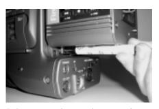
Once mounted, secure the two captive screws at the base of DR-DV5000 to the camcorder.
