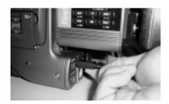
(This may not be necessary on all JVC camcorders. Check with JVC for information on different models. A flexible wire clamp located on the DR-DV5000 base provides restrain for the cable).
