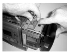
REMOVING THE HDD: Slide the HDD release latch on the DR-DV5000 top plate toward the battery system. Once slid as far as possible, hold the latch while at the same time grasping the FSHDD-1 drive handle and pulling the HDD out from DR-DV5000.
