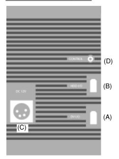
The rear connector panel features a 6-pin FireWire port for DV video I/O (A), a 6-pin FireWire port for connection of external FireWire drives or a computer (B), a 4-pin XLR DC power input (C) and a 3.5mm control cable input for RS232C or GPI (D).
