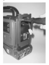
supplied screws). Once "hooked" onto the rear, the 52-pin connector should mount to the equivalent on the GY-DV5000 series. This connector does not exist on other camcorders.
