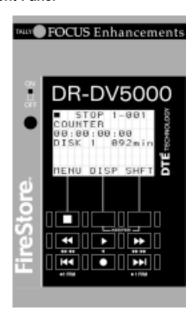
The front panel contains the backlit LCD and 9 buttons for controlling FireStore's functions. The top row of buttons act as soft keys and provide the function displayed on the bottom of the LCD.
