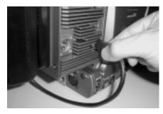
cable from the 6-pin FireWire port on DR-DV5000 marked "DV I/O" to the 4-pin FireWire port on the rear of the camcorder marked "DV"
